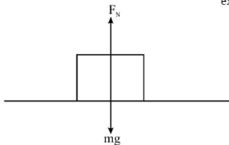
Fig. 4.6 : Normal force on the block
