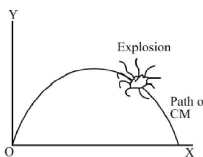
Fig. 6.4 : Centre of mass of a projectile
