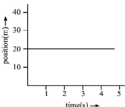
Fig. 2.2 : Position-time graph for a body at rest
