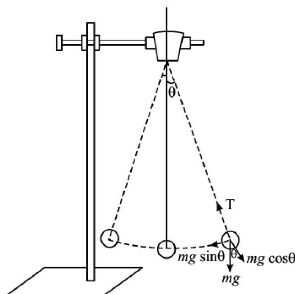
Fig. 7.7: Oscillations of a Simple Pendulum
