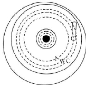
Fig. 6.9 : Pure rotation of a grinding stone
