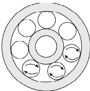
Fig. 4.7 : Balls in the ball-bearing
