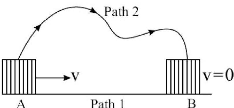
Fig. 5.14 : A block which is given an initial speed v on a rough horizontal surface, moves along a straight line path 1 and comes to rest at B. It starts with the same speed at A but now moves along a different path 2.
