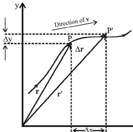
Fig. 3.12 : Displacement  $\Delta r$  and average velocity  $v$
