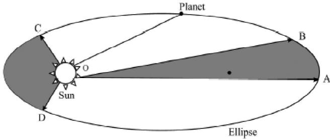
**Fig. 8.9:** The path of a planet is an ellipse with the Sun at one of its foci. If the time taken by the planet to move from point A to B is the same as from point C to D, then according to the second law of Kepler, the areas AOB and COD are equal.
