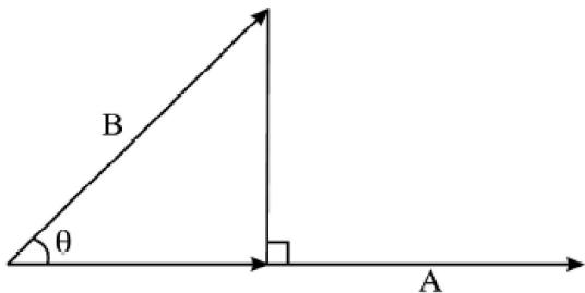
Fig. 3.8 : Projection of B on A
