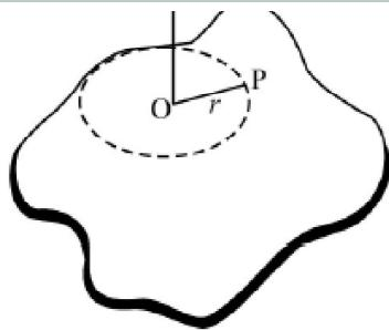
Fig. 6.21 : A rigid body rotating about on axis
