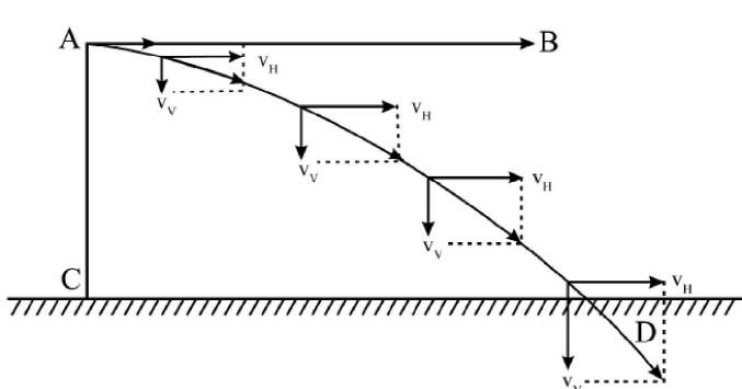
Fig. 3.13 : Curved path of projectile
