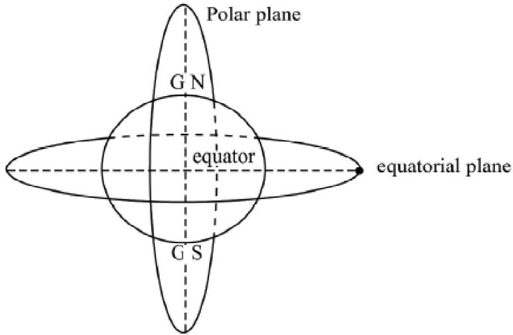
Fig. 8.11 : Equatorial and Polar orbits
