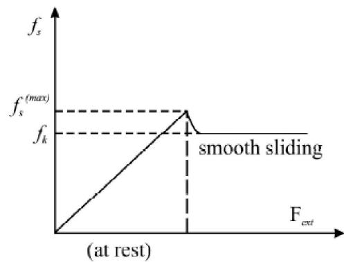
Fig. 4.5 : Variation of force of friction with external force
