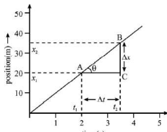
Fig. 2.3 : Position-time graph for uniform motion
