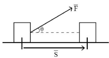
Fig. 5.1 : Work done in moving a block by applying a Force  $\bar{F}$  by a displacement  $\bar{S}$
