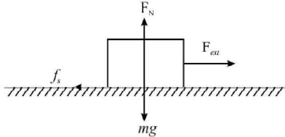
Fig. 4.4 : Forces acting on the block
