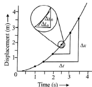
Fig. 2.5 : Displacement-time graph for non-uniform motion
