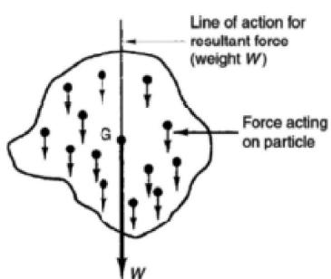
Fig. 6.6 : Resultant weight acting along the centre of gravity
