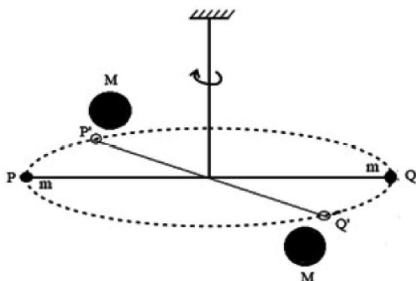
Fig. 8.3 : Schematic drawing of Cavendish's
