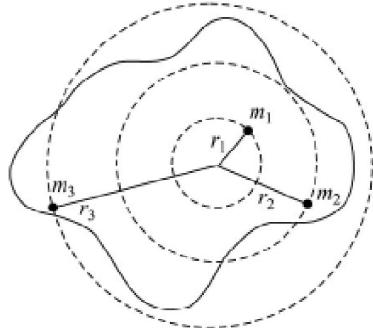
Fig. 6.12 : Rotation of a plane lamina about an axis passing through its centre of mass
