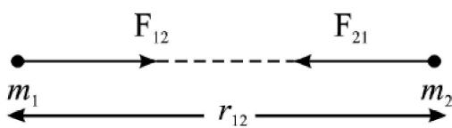
Fig. 8.2 : The masses  $m_1$  and  $m_2$  are placed at a distance  $r_{12}$  from each other. The mass  $m_1$  attracts  $m_2$  with a force  $F_{12}$  and the mass  $m_2$  attracts  $m_1$  with a force  $F_{21}$ .
